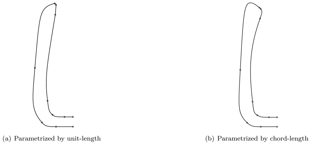
Figure 8: Profile of vase using G^2 cubic Bézier spiral transition curves.
